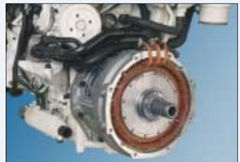
DC integrated flywheel starter motor generators for hybrid drives
